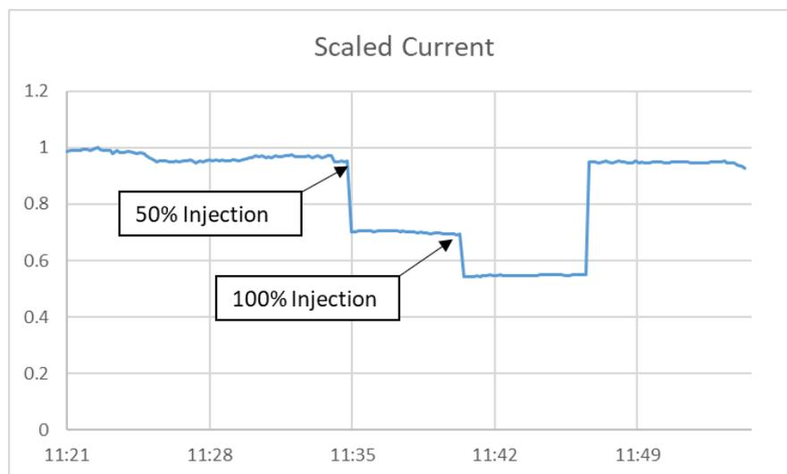
Figure 3: Scaled Current in line P20 during Manual Injection
