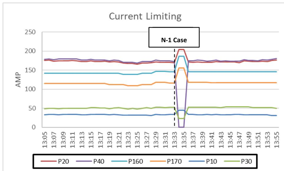
Figure 4 - Line Current during the N-1 Contingency Case
