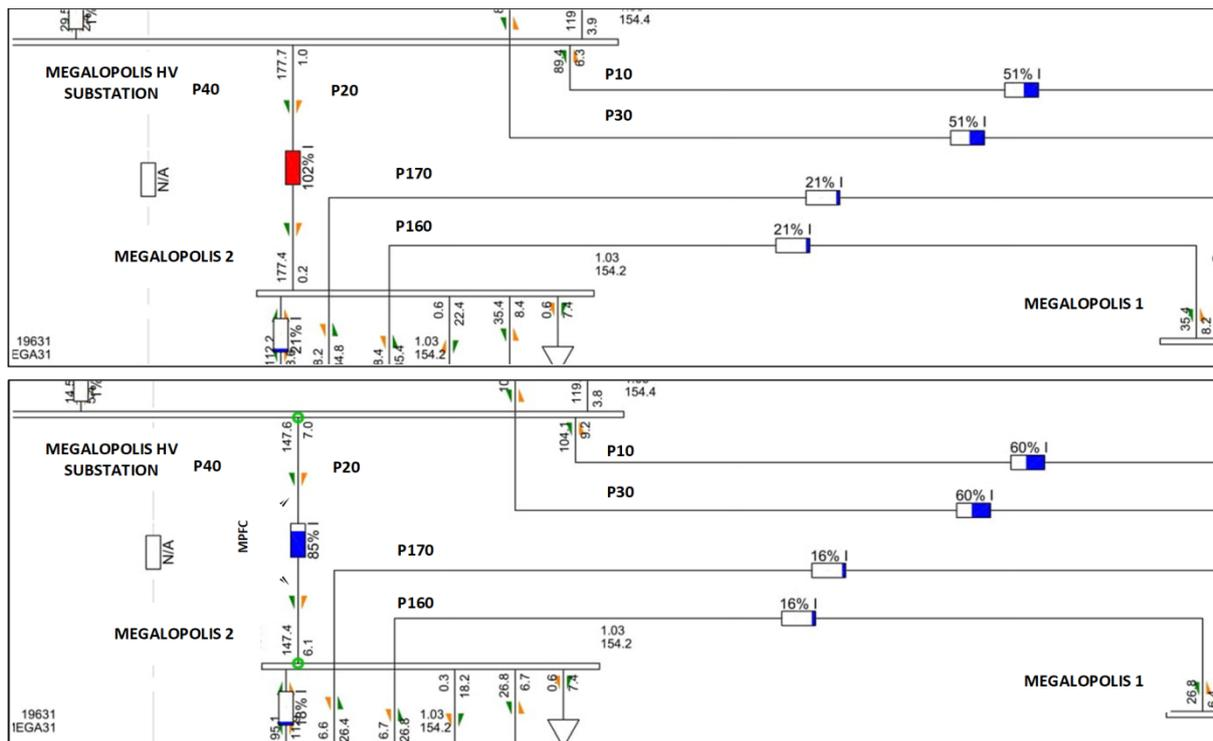
Figure 1 : N-1 contingency without (top) and with (bottom) the mobile MPFC device installed. The installation of the mobile MPFC device resolves the overload by redirecting power flows to adjacent transmission lines.
