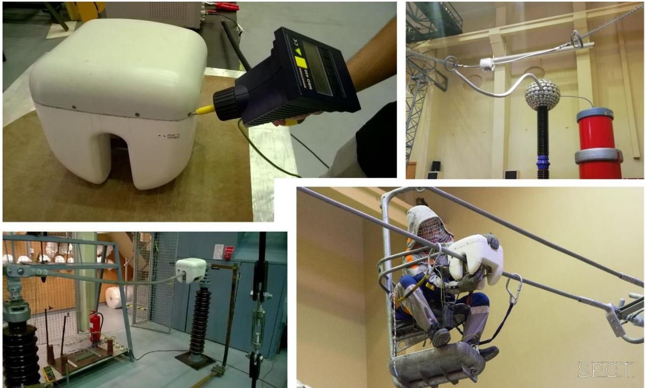
*Figure 1 - Sensor tests were performed on the OTLM line monitoring device at BME's High Voltage Laboratory*
