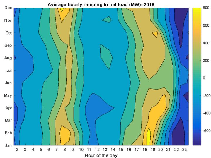
***Average hourly ramping up in net load for 24 h (2018).***
