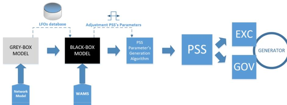
The grey-box model, which takes into consideration the network model of the power system, analyses the system's dynamics for multiple scenarios in order to identify potential LFO modes that could be activated. This analysis generates a database of simulations that will be used by the black-box model to complement the training process of the data-driven algorithm.
